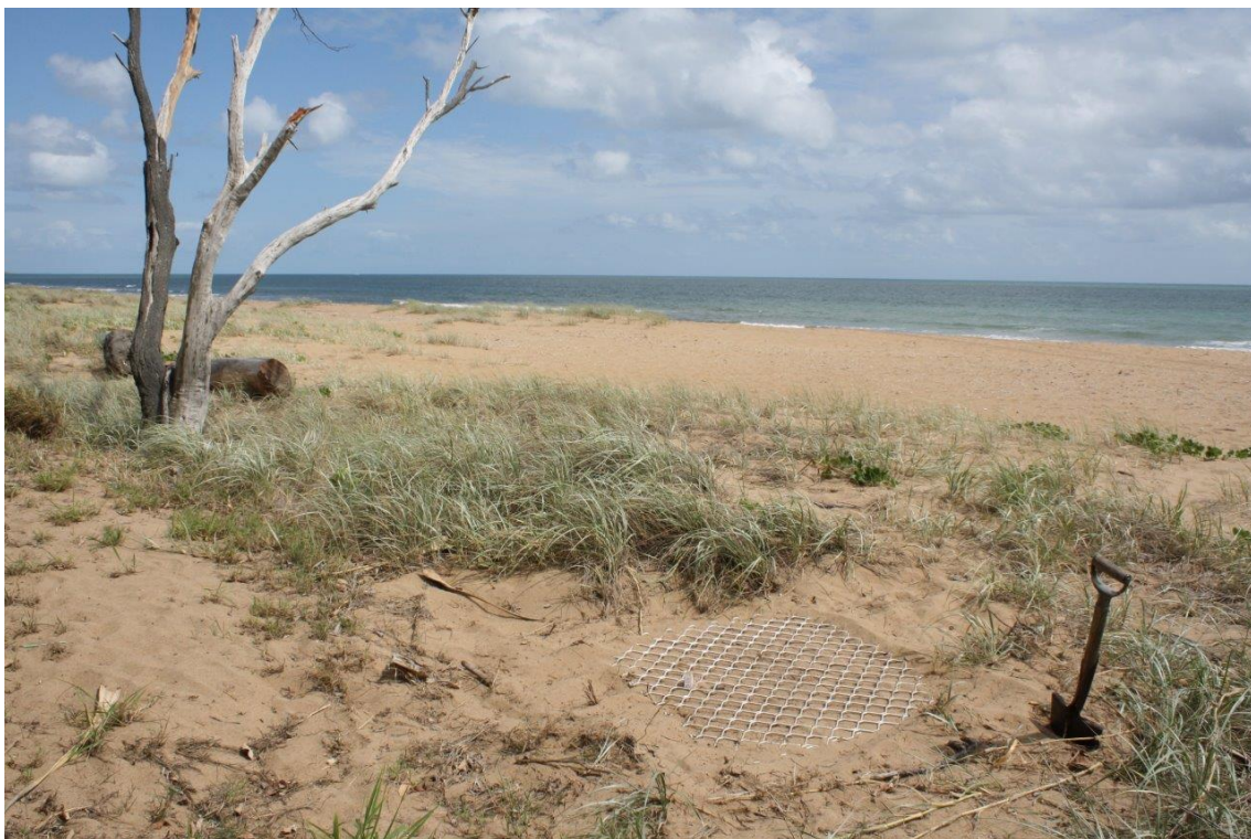
Figure 2. A flatback turtle clutch protected from vertebrate depredation of the eggs by placement of an aluminium mesh Predator Exclusion Device (PED: 1 m x 1m with 30 cm buried vertical walls and 70 mm diameter meshes) on Moore Park Beach.
