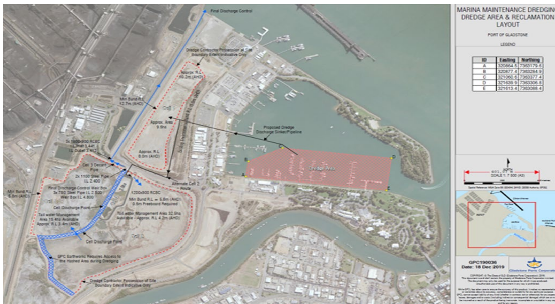
Figure 1 Marina Dredge Footprint and RGT Reclamation Area
