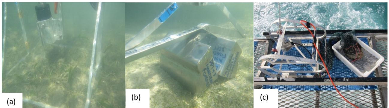
Figure 2. Seagrass monitoring methods used in the Port of Bundaberg in 2020. Boat-based camera drops (a) and van Veen grab (b) for subtidal seagrass and video sled (c) used to sample deep-water seagrass.
