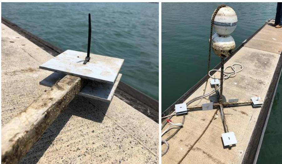
Figure 5: Settlement array setup for surveillance event 2, showing plate 'sandwich'
