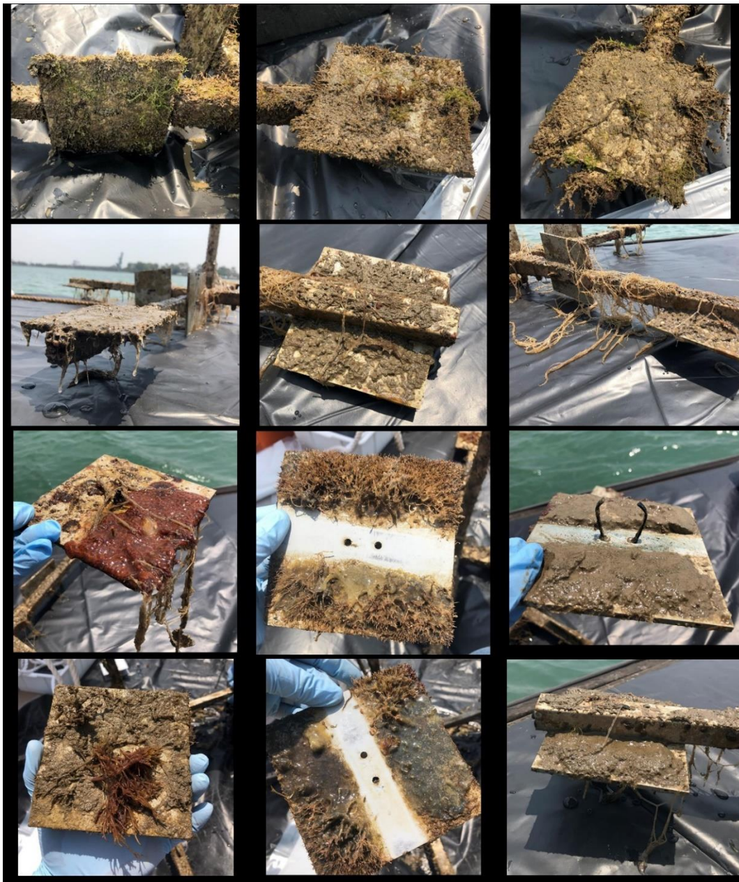
Figure 12: Representative settlement array fouling at the Port of Gladstone (event 1)
