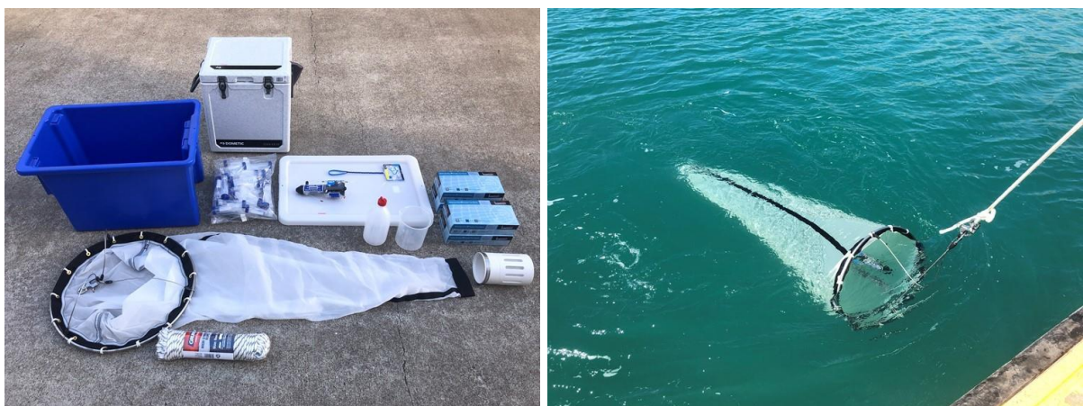
Figure 7: Plankton sampling equipment kit
