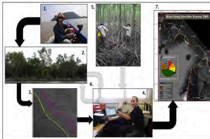
Fig. 1. Schematic diagram showing the steps involved in the shoreline video assessment method (S-VAM). 1. Image acquisition 2. Image processing 3. Image geolocation 4. Image classification 5. Filed plot validation and groundtruthing results. 6. QAQC 7. Mapped output and data visualization.
