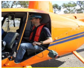
Figure 5: Camera staff as used in helicopter (installed below helicopter skids after take off).
