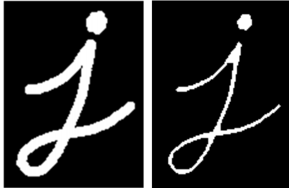
Supplementary Figure 10: Left: Original binary image. TRUE or 1 is represented by white, and FALSE or 0 by black. Right: Image after an erosion filter with an SE as a 5x5 pixel box is applied.
