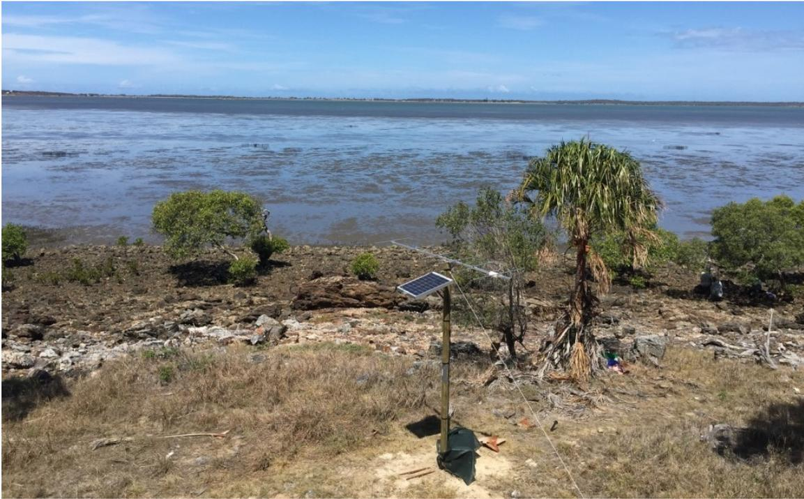
**Figure 5.5** Example of an automatic radio-tracking station on Curtis Island, set on an elevated position (to increase detection range) overlooking Pelican Banks.
