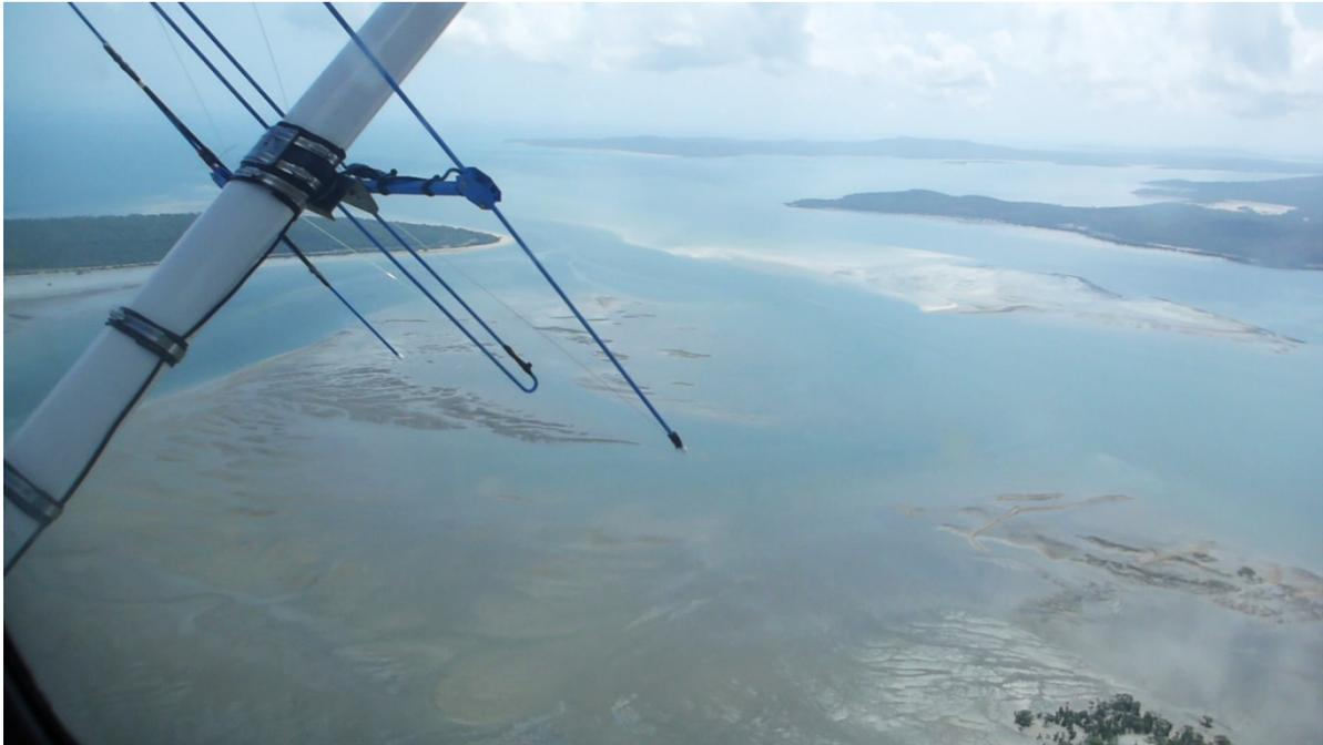
**Figure 5.7** Aerial tracking over the exposed intertidal flat in the Rodds Peninsula subregion. The 3-element Yagi antenna was attached under the wing of the aircraft to improve the reception of radio signal.
