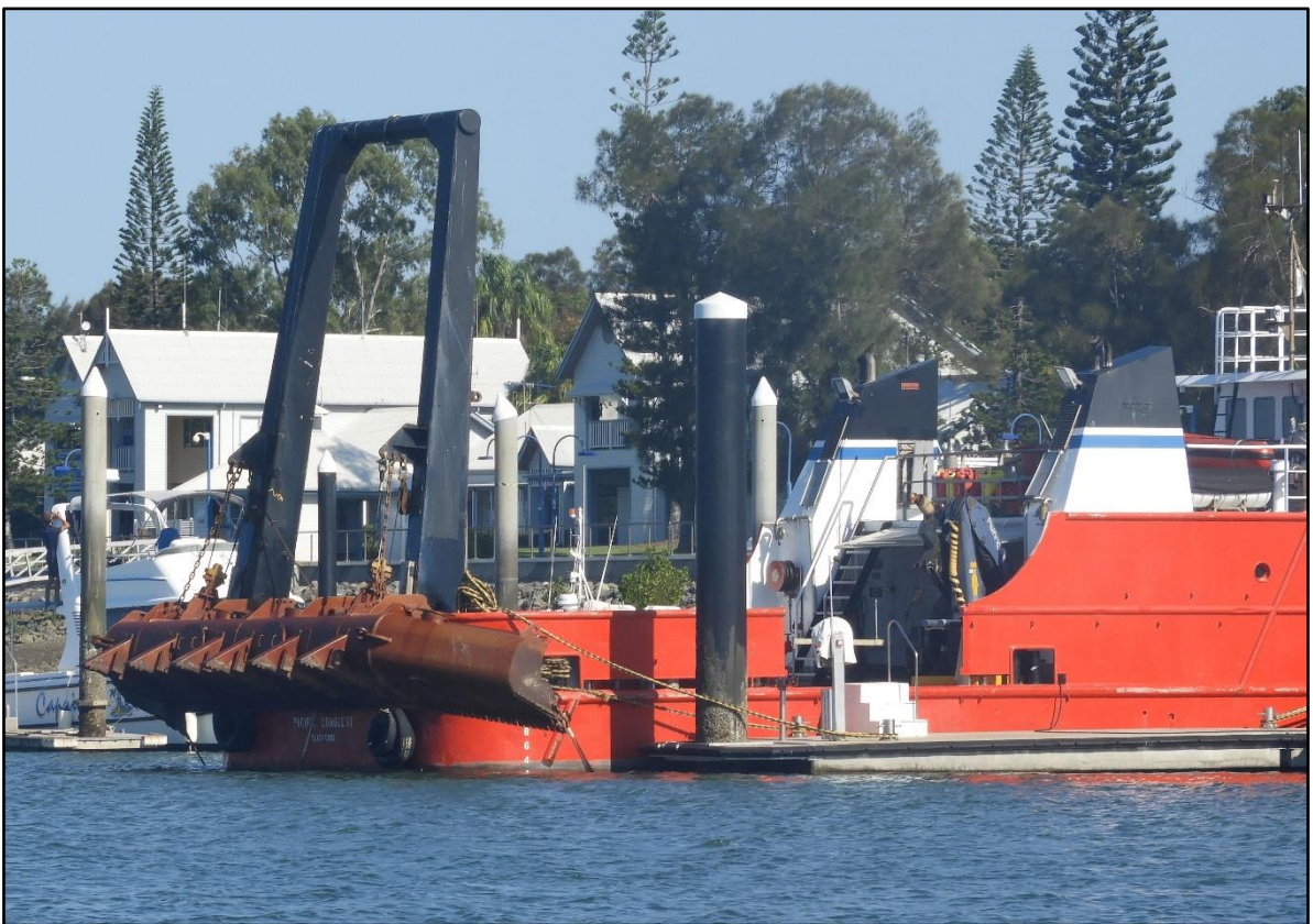
Figure 5-5 A dredge channel maintenance vessel in Gladstone Marina, February 2018. The blade on the stern of the vessel is deployed in the dredge channels a bit like a grader blade (Adam Leavesley, Wildlife Unlimited).
