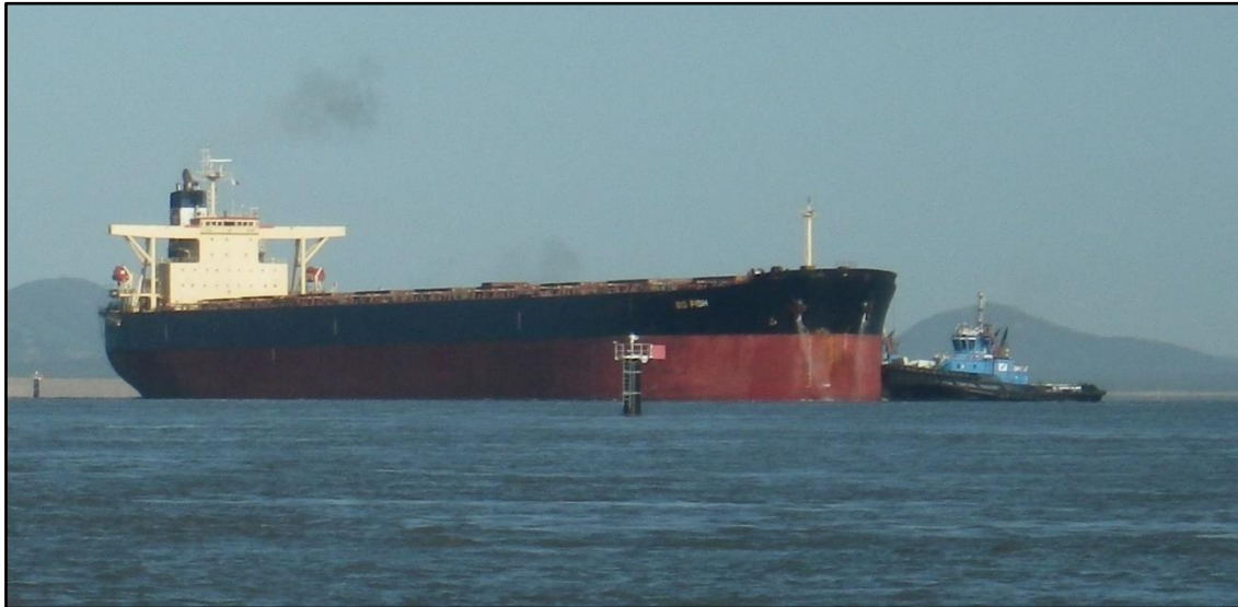
Figure 1-2 The swing basin at the Wiggins Island Coal Export Terminal (WICET), February 2018 The vessel is the Big Fish, a 177,662 dwt Capesize bulk carrier registered in the Marshall Islands. Capesize ships are so named because they are too big to traverse the Panama Canal (Adam Leavesley, Wildlife Unlimited).
