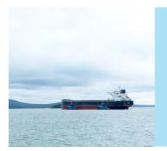
Large ships with the bridge at the stern will have a large blind spot for several hundred metres in front of the bow. This blind spot extends much further forward if deck cargo or containers are carried.
