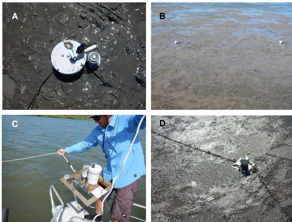
Figure 1. Dual Odyssey BPAR loggers and wiper units were deployed on stakes in the sediment (A & B) and on deployment cradles connected to surface floats (C & D).
