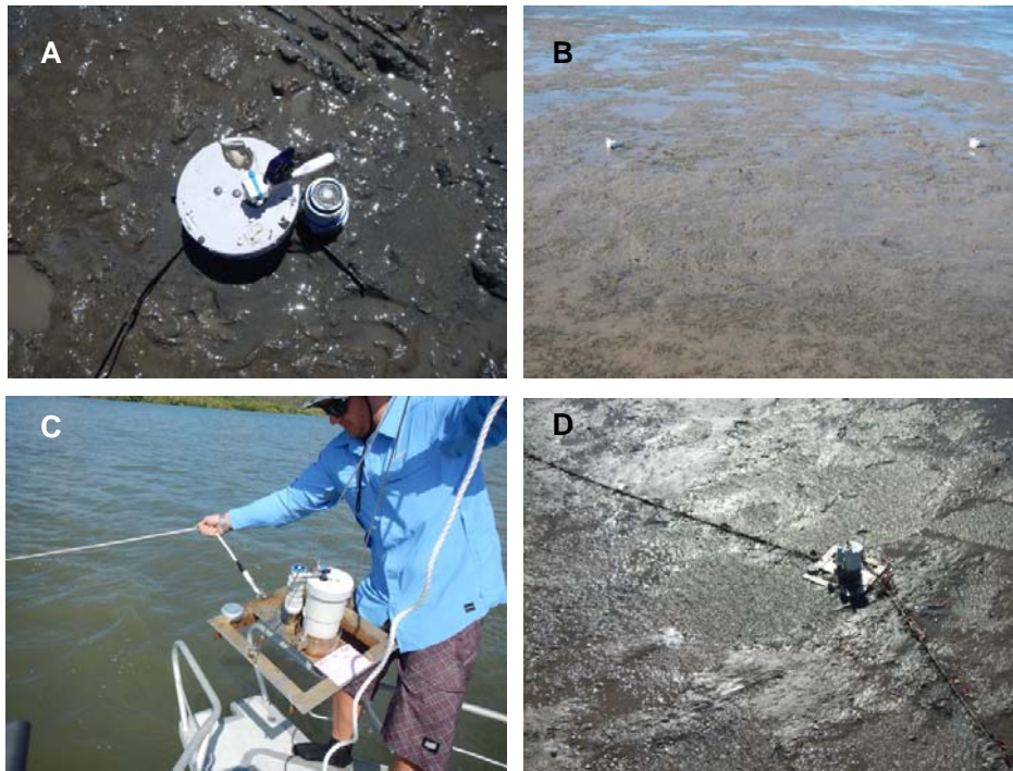
Figure 1. Odyssey BPAR loggers and wiper units deployed on stakes in the sediment (A & B) and on deployment cradles connected to surface floats (C & D).
