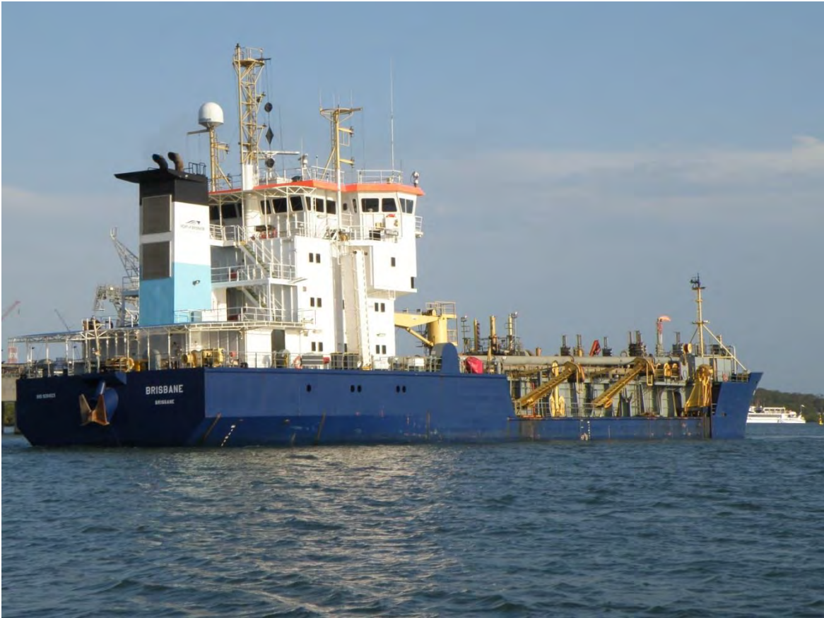
Figure 1-1 TSHD Brisbane Dredging in APLNG Swing Basin
