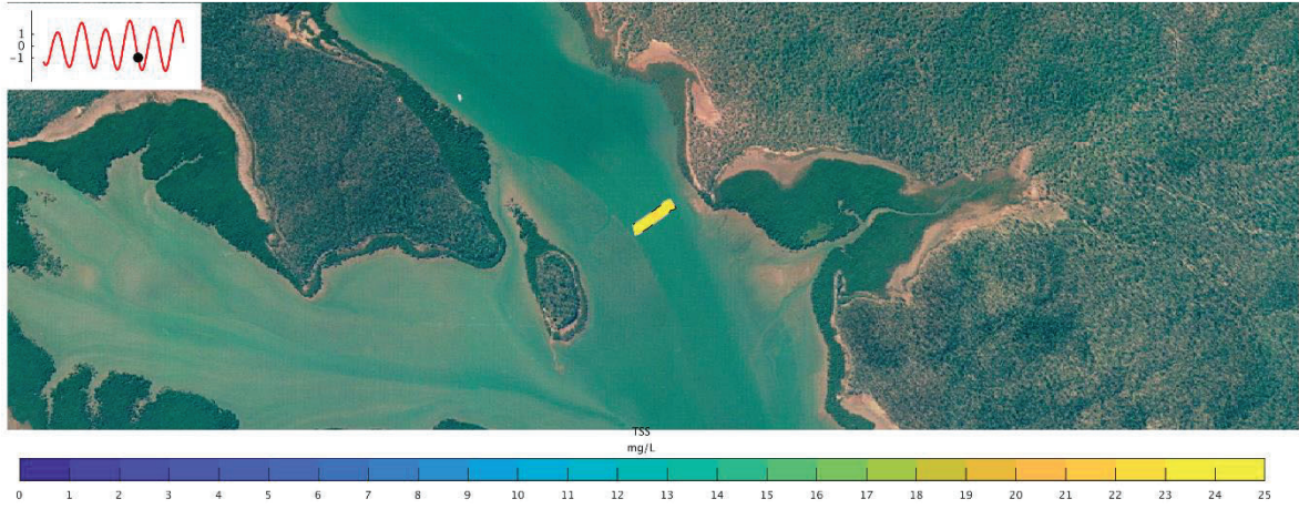
Transect of Dredge Plume in Plan
