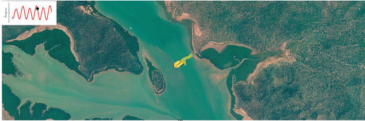
Transect of Dredge Plume in Plan
