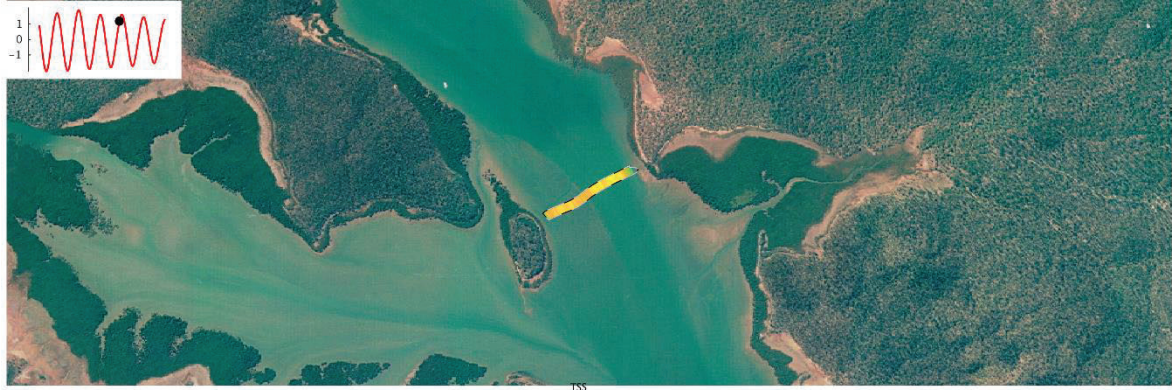
Transect of Dredge Plume in Plan
