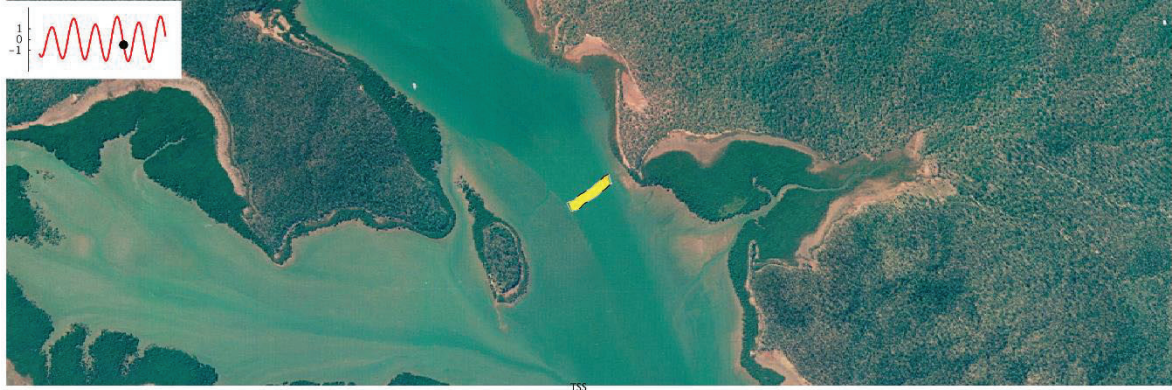
Transect of Dredge Plume in Plan
