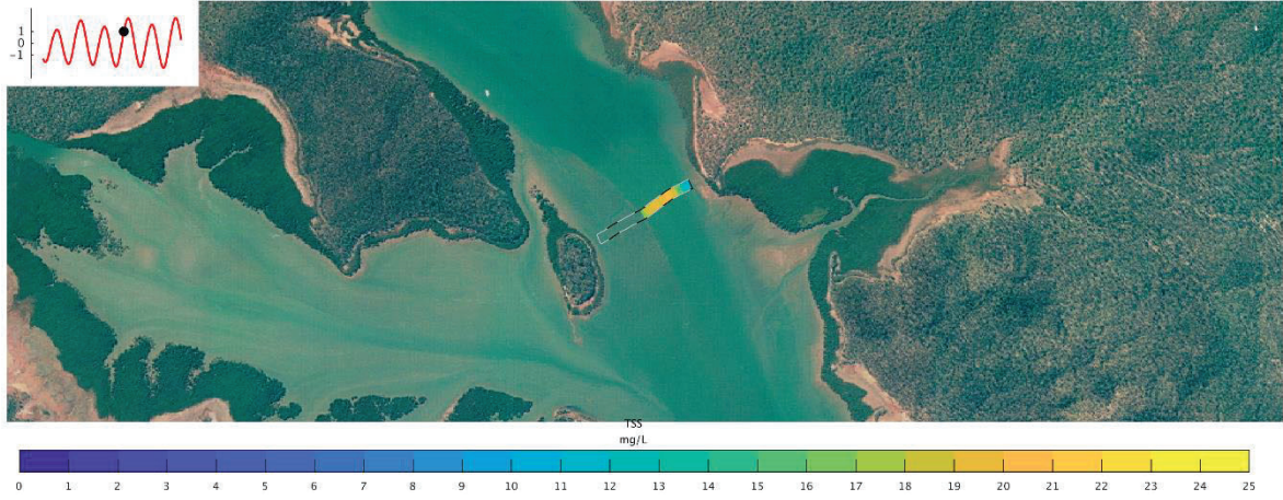
Transect of Dredge Plume in Plan
