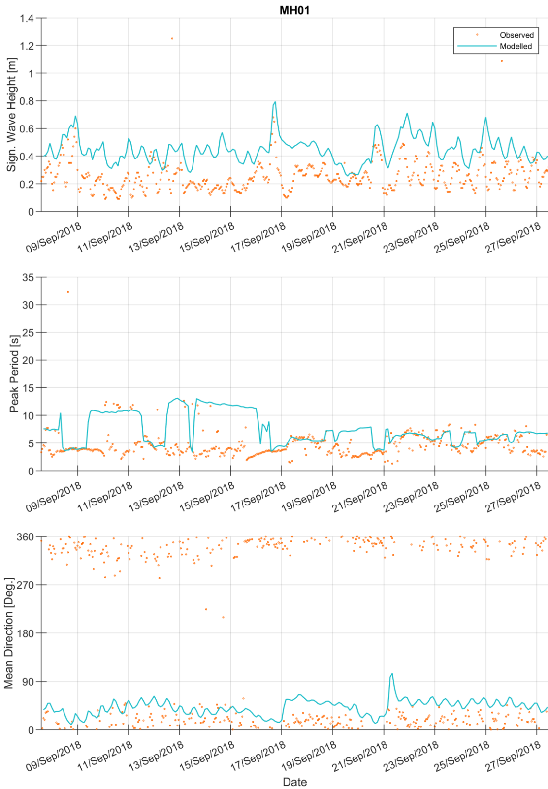
Figure B-5 Timeseries comparison of modelled and observed Wave Height (Top), Peak Period (Centre) and Peak Direction (Bottom) at MH01
