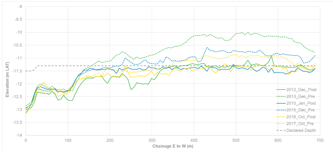
Figure 25. Historic bathymetry along Auckland Pt Berth1 transect.
