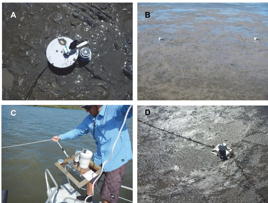
**Figure 1.** Dual Odyssey BPAR loggers and wiper units deployed on stakes in the sediment (A & B) and on deployment cradles connected to surface floats (C & D).
