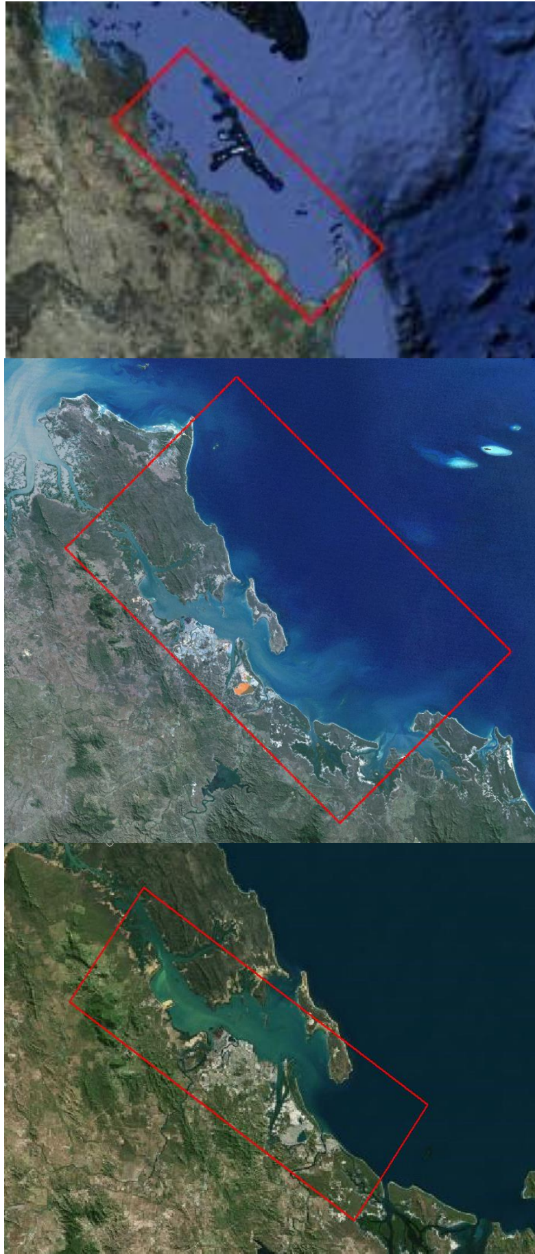
Figure 2-2 SWAN Wave Model Domains (GBR domain – Top, Regional Domain – Middle, Local Domain – Bottom)
