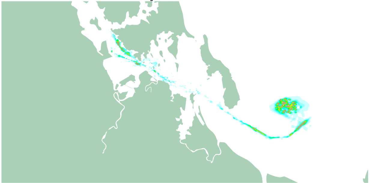
340000m 3 Campaign - Impact of dredging on the 95th %ile of deposition rate 10-Aug-2017 00:00 to 01-Oct-2017 00:00
