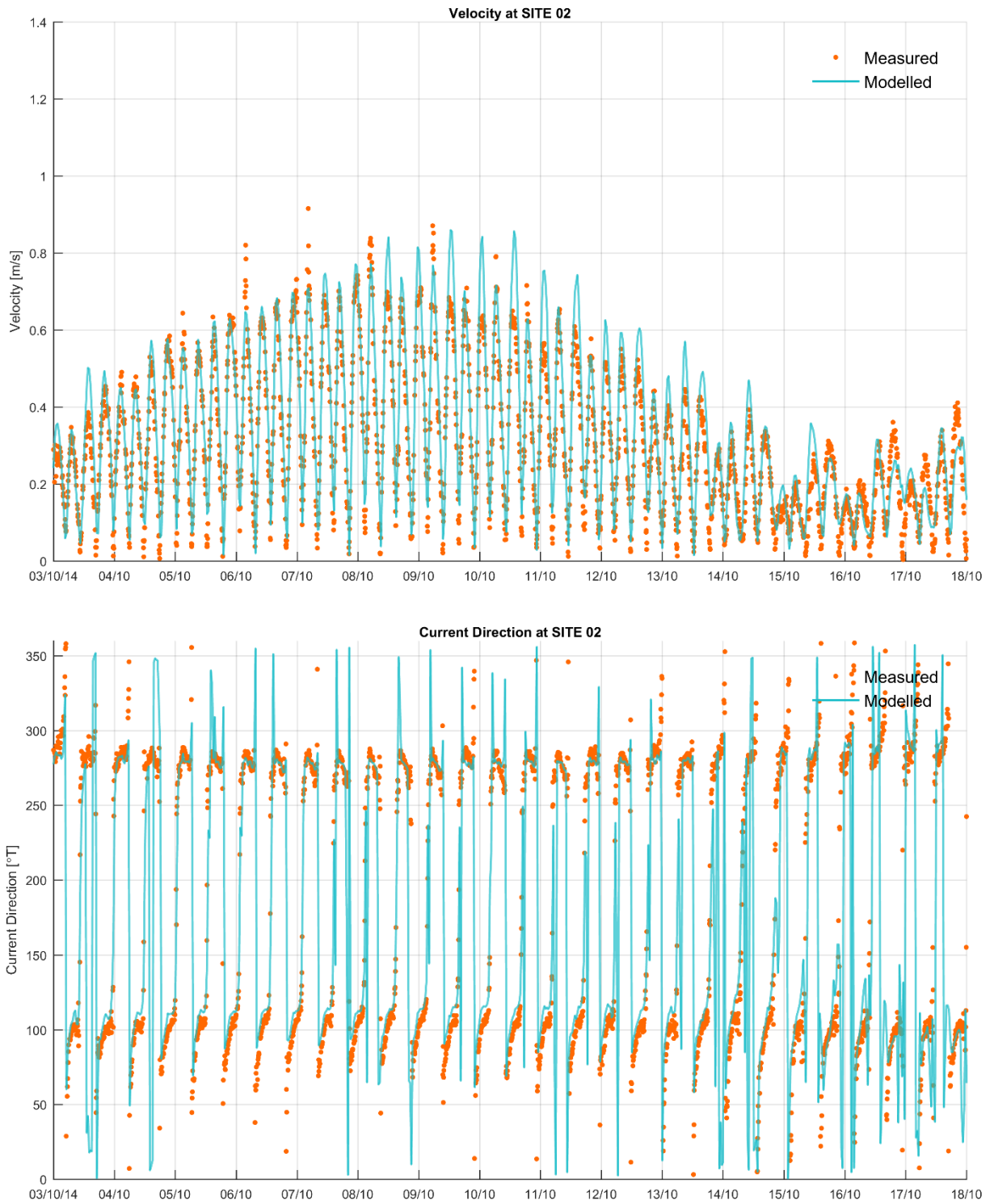
Figure 5-5 Modelled (Solid Line) and Measured (Dots) Depth-Averaged Current Velocity at Site 2
