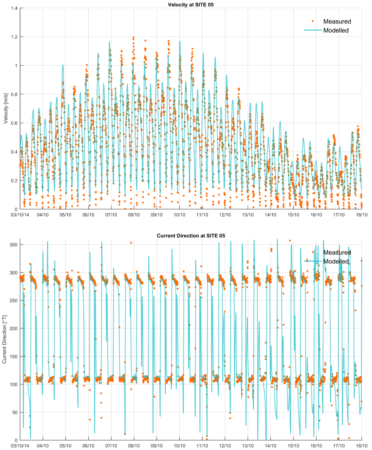
Figure 5-8 Modelled (Solid Line) and Measured (Dots) Depth-Averaged Current Velocity at Site 5
