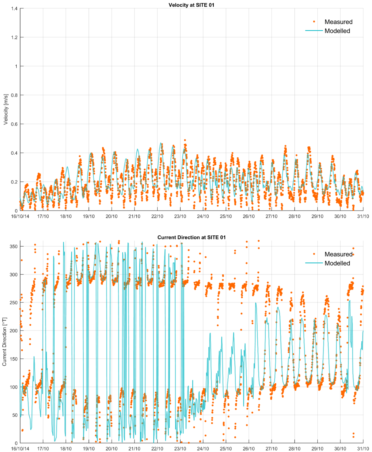
Figure 5-4 Modelled (Solid Line) and Measured (Dots) Depth-Averaged Current Velocity at Site 1
