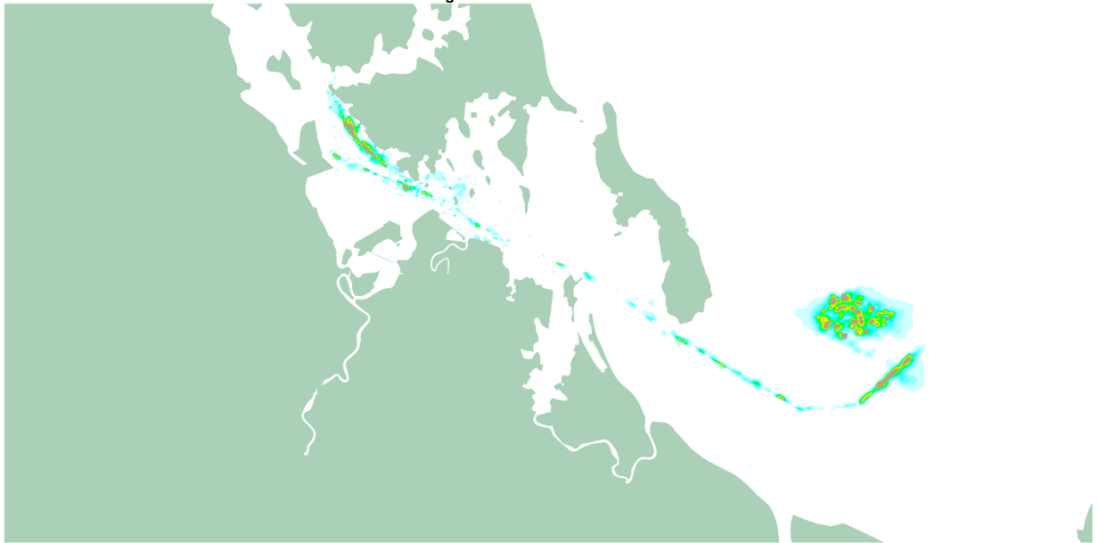
300000m 3 Campaign - Impact of dredging on the 95th %ile of deposition rate 10-Aug-2017 00:00 to 01-Oct-2017 00:00
