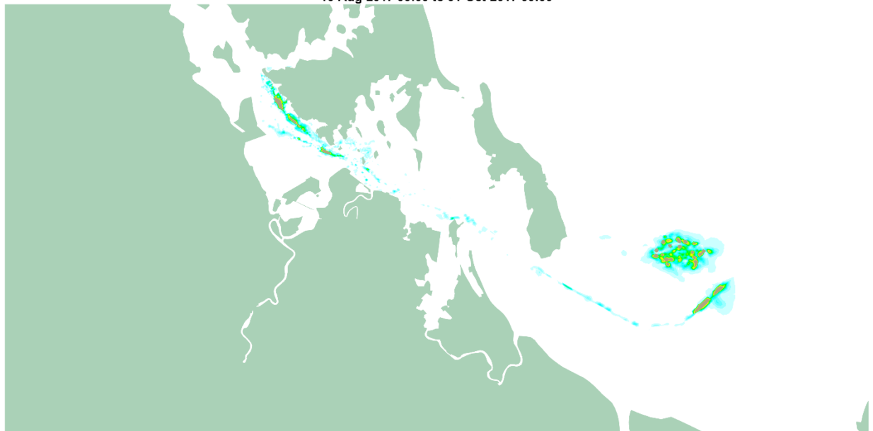
220000m 3 Campaign - Impact of dredging on the 95th %ile of deposition rate 10-Aug-2017 00:00 to 01-Oct-2017 00:00
