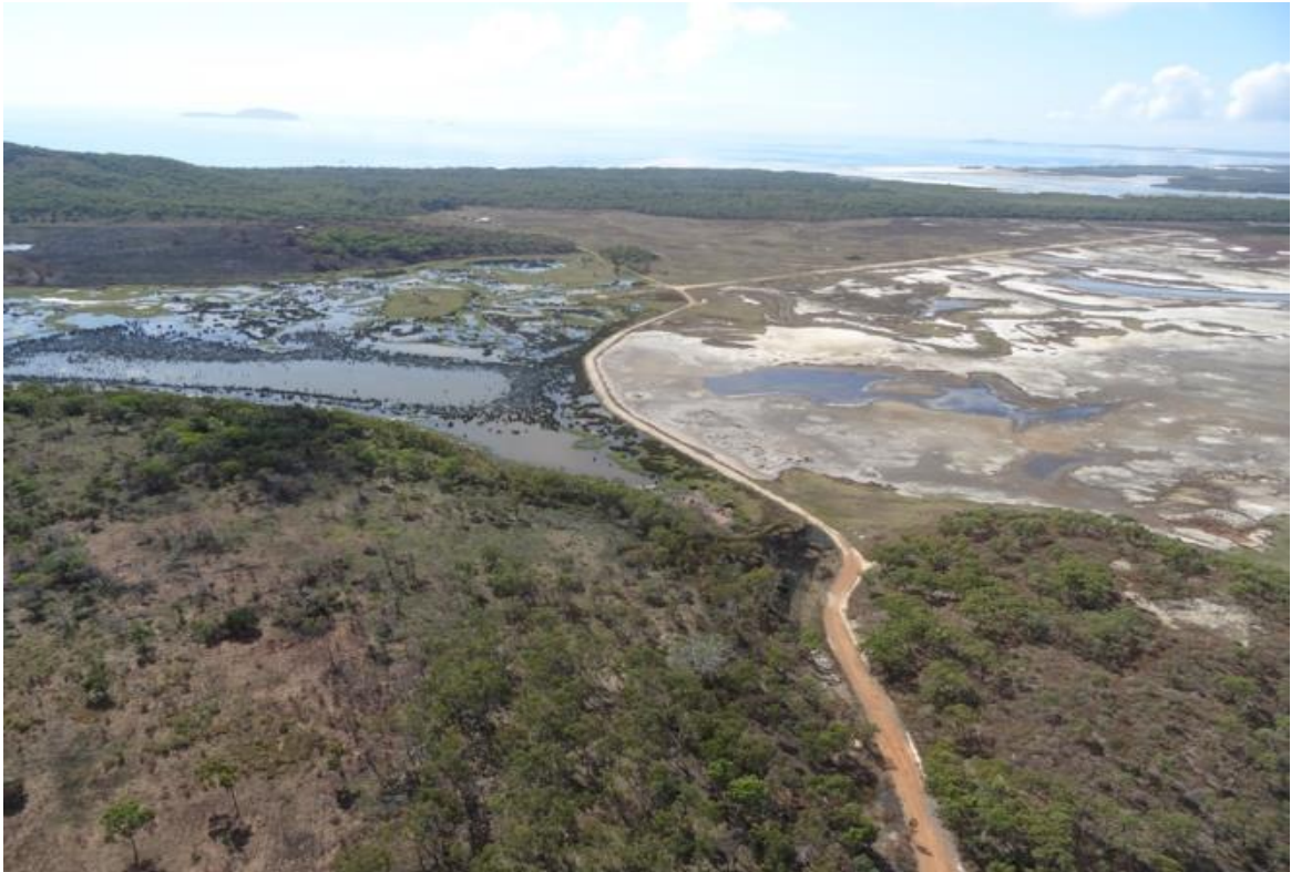
Figure 61. Human altered hydrology caused by construction of drainage channels through tidal wetlands. The example from the north end of Curtis Island, identified a road on an earthen bund cutting across a tidal area. Because of inadequate drainage, the upper area has trapped extensive tidal areas, causing excessive ponding with the death of impounded vegetation. Such damage is entirely avoidable and it is easily managed by installing more considered and open drainage under the road. This type of impact should be easily fixed by improving drainage under the road. (Source: NC Duke).
