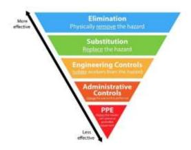
Figure 2: Hierarchy of control model
