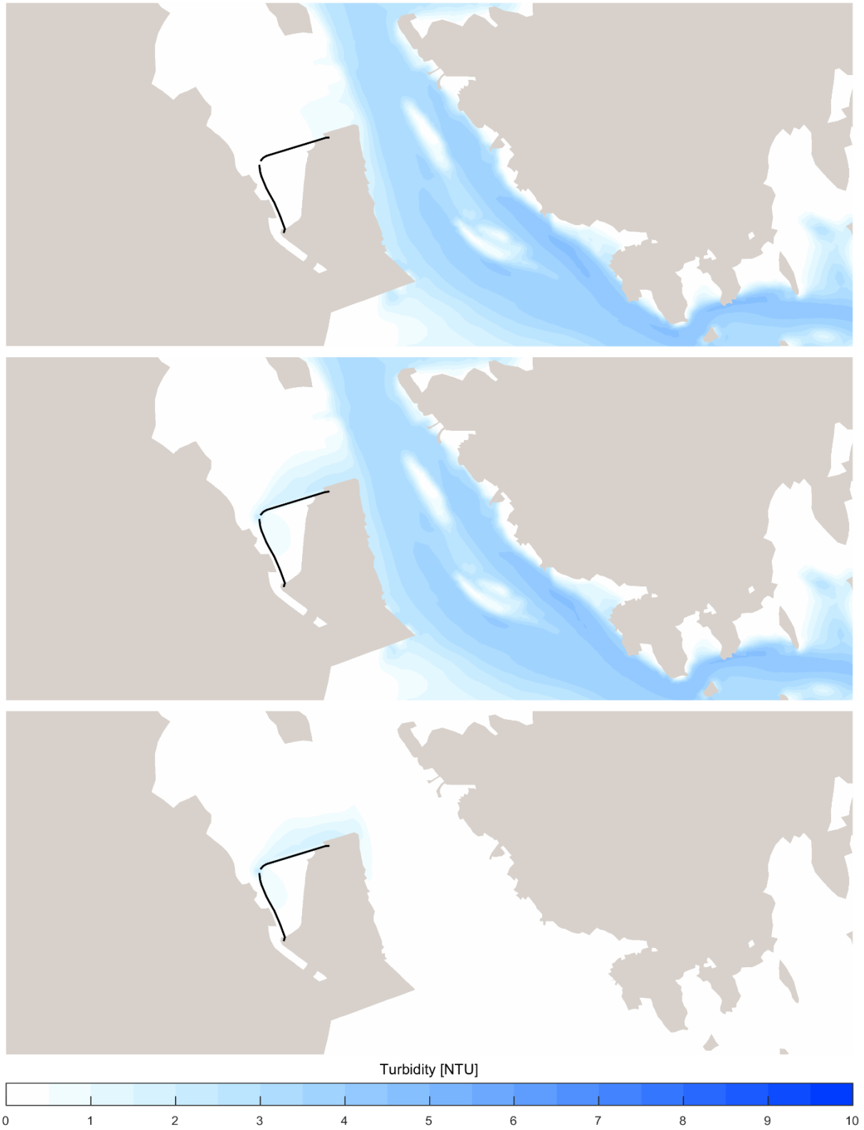
Figure 31 Scenario 1C (12-hr Construction Operations). 50 th Percentile Turbidity Base Case (Top), With Construction (Middle) and Difference (Bottom)
