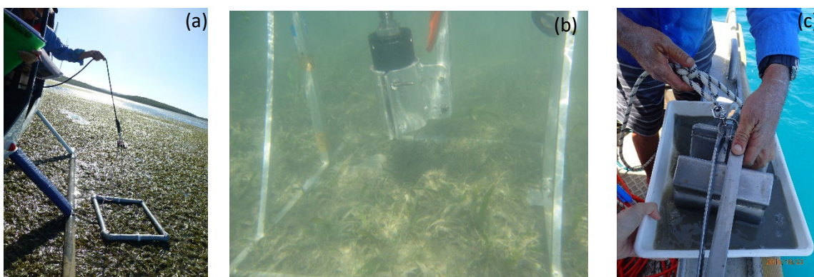
Figure 6. Seagrass monitoring methods in 2023. (a) helicopter survey of intertidal seagrass, (b, c) boat-based camera drops and van Veen grab for subtidal seagrass.
