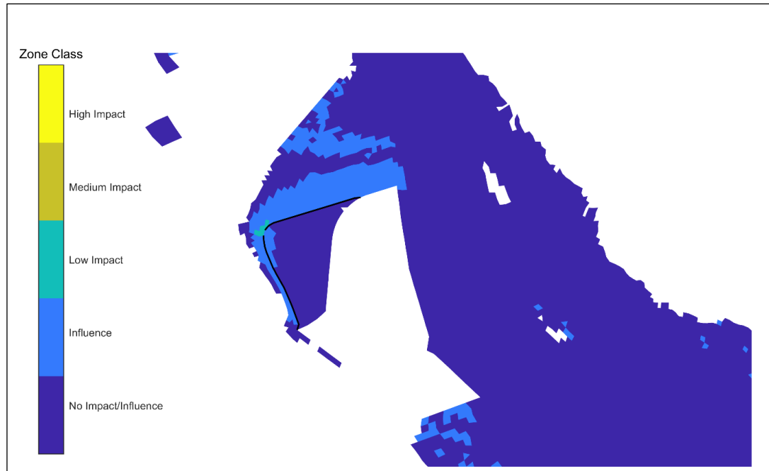
Figure 12: ZOIs and Zone of Influence for Scenario 1C, prior to bund closure, 12 hours operations
