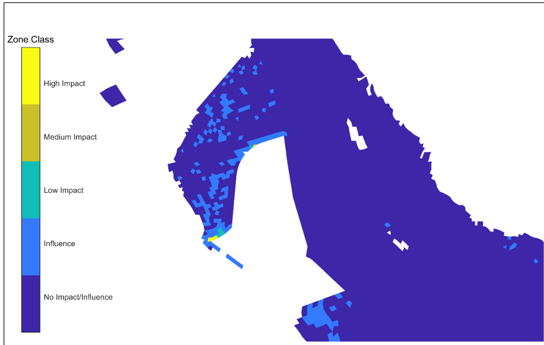
Figure 8: ZOIs and Zone of Influence for Scenario 1A, start of bund construction, 12 hours operations
