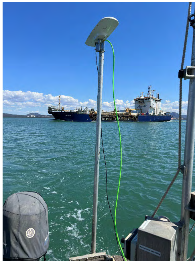
Figure 1.7 TSHD Brisbane whilst steaming out laden. ADCP mounting pole and GNSS in foreground
