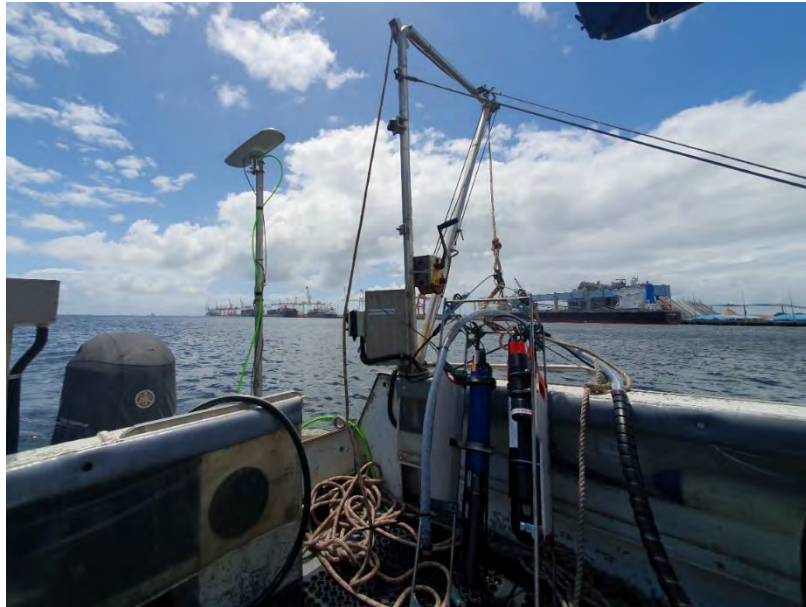
Figure 2.1 Plume monitoring equipment setup including the GNSS and ADCP mounting pole, and the profiling array including the co-located LISST, YSI and pump sampler frame.
