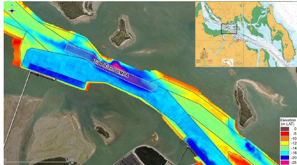
*Note: if it is assumed that 75,000m<sup>3</sup>/yr is placed at Tide Island DMPA instead of EBSDS this would reduce dredge time from 10 days to 4.3 days and cost from \$990,000 to \$430,000.*
